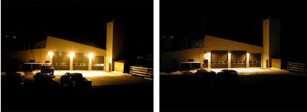
Figure 3. Shielded light fixtures at a commercial docking facility. Source: Intro to Lighting PowerPoint. (2017). IDA. Retrieved from: <http://darksky.org/resources/public-outreach-materials/#pp>
